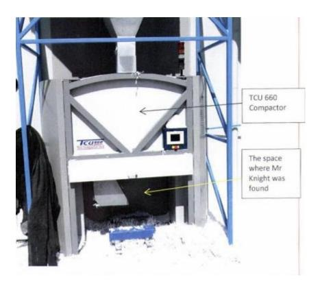
From the time the paper trim extraction unit was installed, and the CU connected by way of the locally manufactured chute from the large collection hopper the rams of the CU became blocked by paper trim which caused the CU to stop working.<sup>24</sup> As to why this occurred the manufacturer of the trim extraction unit, Integrated Air Systems, advised WST of the following:
